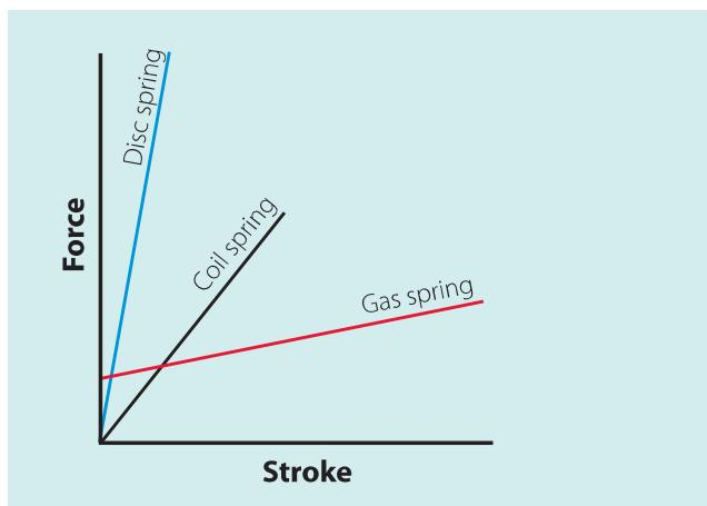
As the piston rod is pressed into the tube, volume reduces and pressure increases. This causes pushing force to increase. In conventional gas springs, this increase is normally around 30% at full compression.
