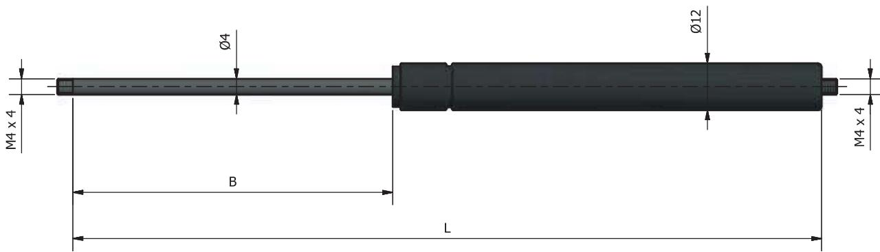
**Gas spring with pneumatic extension speed ~0,3 m/s**
