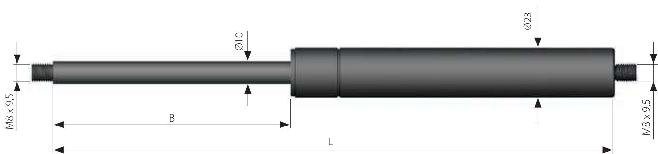
**Conventional gas spring with extension speed ~ 0.3 m/s**
