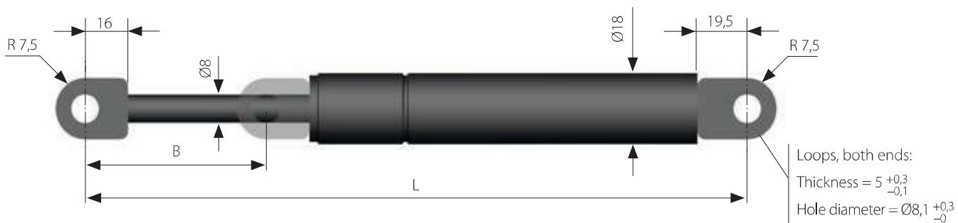
**Conventional gas spring with welded loops, extension speed ~ 0.3 m/s**
