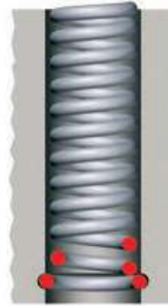
4. Enlarged end coil for mounting in groove
