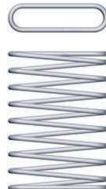
9. Rectangularly wound compression spring (magazine spring)
