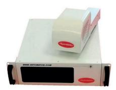
MOPA<sup>II</sup> comes with three main components: the BOX contains the source and the electrical components, The HEAD with a galvanometer for fast x/y movement and focal lens and the FIBER optic cable that connects the two. The AUTOMATOR MOPA<sup>II</sup> couples the stability of a fiber laser with our proprietary EuGENIUS<sup>TM</sup> software to create market leading "power-to-the-part" performance.
