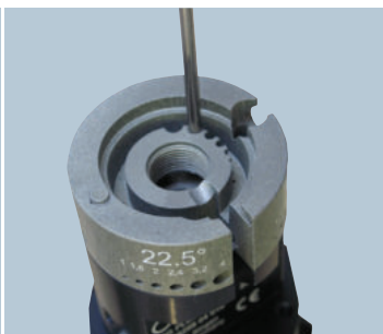
Squaring an electrode tip
