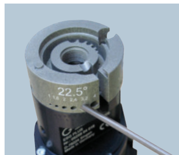
Grinding electrodes: - 4 different angles, 6 different electrode diameters
