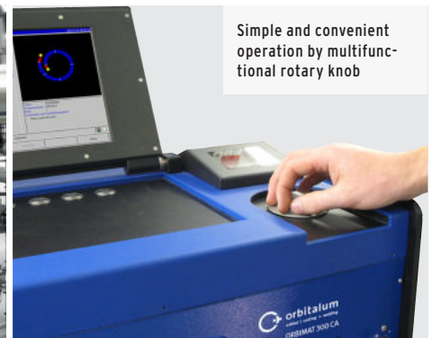
10.5" swivel monitor and system printer integrated
