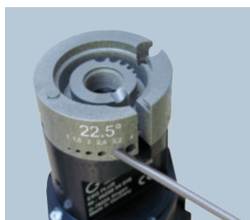
Grinding electrodes: - 4 different angles, 6 different electrode diameters
