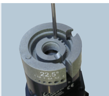
Squaring an electrode tip
