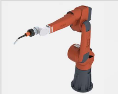
QRH-360/390-H Wrist with hollow shaft, high robot base
