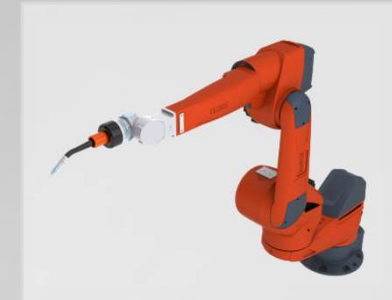
QRH-360/390-E Wrist with hollow shaft, with 7th axis
