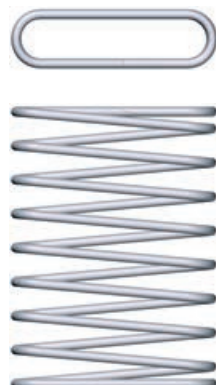
9. Rectangularly wound compression spring (magazine spring)
