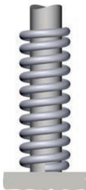
2. Not ground with internal location
