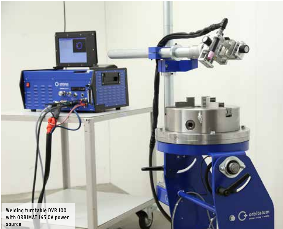
Three-jaw chuck for exact positioning and fixating of the workpiece
