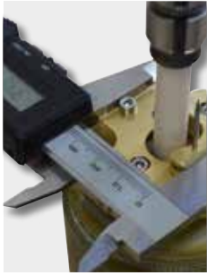
Simple and precise setting of the electrode position
