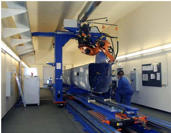
With the new CLOOS robot laser welding system Manitowoc moves into state-of-the-art production technology. The top and bottom of the auto crane boom sections which measure up to 14 m (max. 19 m) are welded and drilled on the system.
