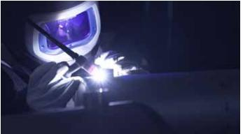
Photo 3: Beside the automated welding technology, Heun uses 22 welding machines for manual MAG and TIG welding.
