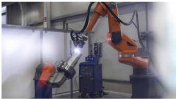
Photo 5: A CLOOS QIROX robot uses the TIG Weld process to weld circular welds for tank containers.
