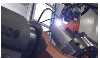
Photo 6: In the past, it took 25 minutes to weld the tank containers manually, now the robot only needs 12 minutes to weld the same component.
