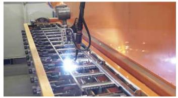
Photo 4: The 2-station design allows loading and welding at the same time.
